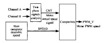
Fig. 8. Design flow diagram of motor feedback controller
