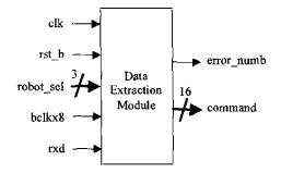
Fig. 5. Block diagram of the data extraction module.
